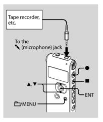
You can make music files without using the computer by recording the sound from other equipment connected to the IC recorder.
